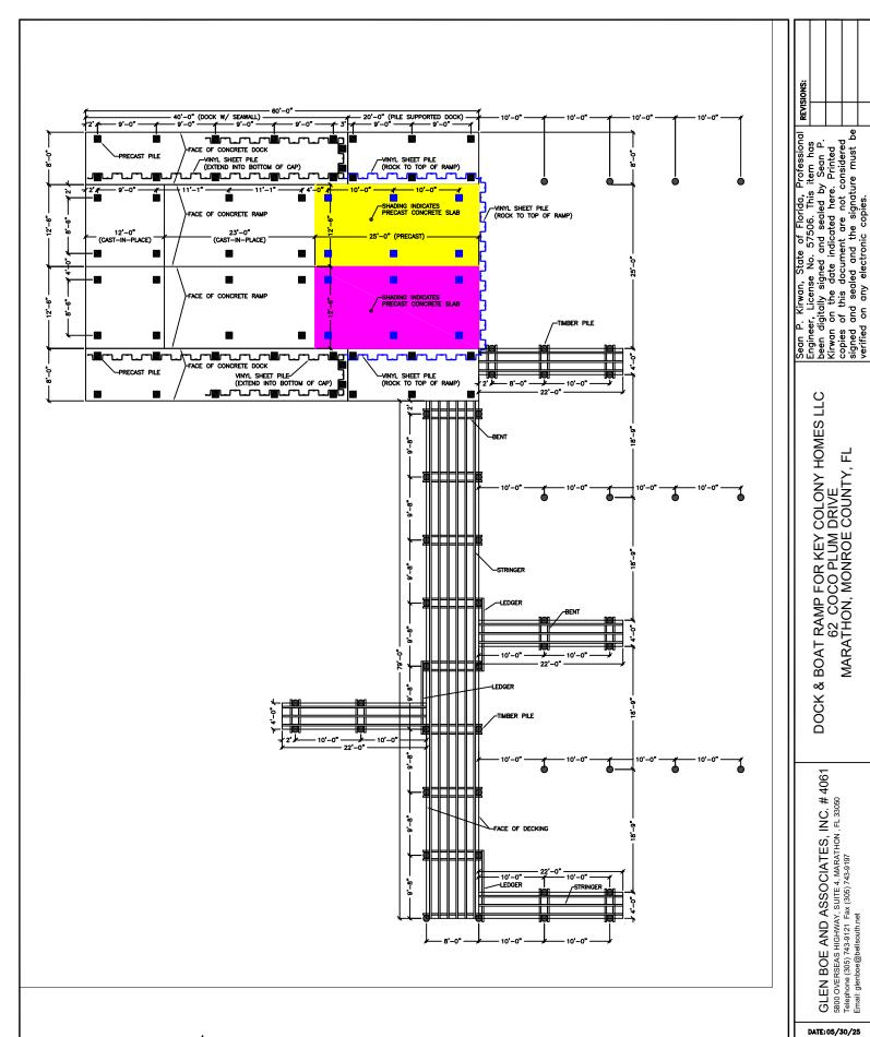
FOUNDATION/FRAMING PLAN SCALE: 1/16" = 1'-0"
